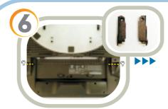
Secure the left and right accessory covers to the unit using two screws from the Speaker Bar/Scanner kit. Note: If installing the Speaker Bar/Scanner on an ESY17A2 or ESY15A2 touchcomputer, skip steps 7-9
