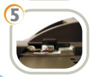
Insert the connector of the cable (both of right and left) accompanying the scanner into the mating connector on the accessory hub in the side of the unit.
