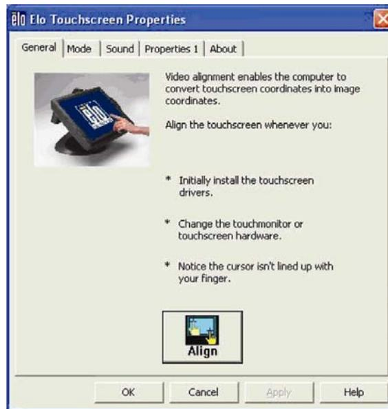
Click the **Align** button. This launches the calibration program. The window shown below opens. Follow the instructions to calibrate the touchscreen.
