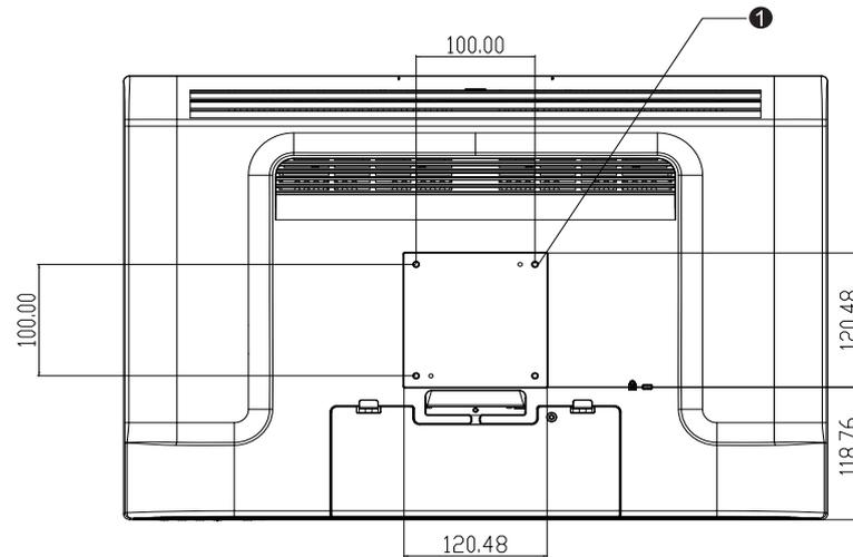
*Figure 2-1 : VESA mounting interface location, pedestal removed*
