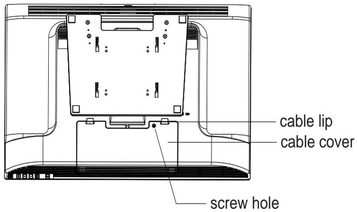
Then you have attached all the cables to the monitor, gently bring all the cables toward the standard so they fit under the cover lip. Remove the screw from accessory and insert the screw into cable cover. Snap the Cable cover in place over the connections.
