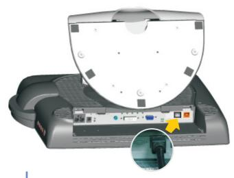
Remove the rubber cap labeled "MSR" from the left USB connector and discard. Connect the USB cable from the MSR kit to the USB connector.
