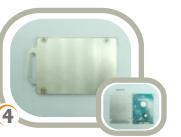
Remove the hard drive caddy from Grasp the handle of the hard drive and push the hard drive into the slot the old hard drive and mount it onto the new hard drive. with the manufacturer's label facing up. Push the hard drive into the slot
