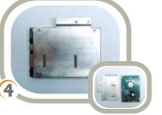
Remove the hard drive caddy from the old hard drive and mount it onto the new hard drive.
