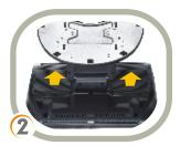
Carefully place the touchcomputer facedown on a soft, flat surface. Turn touchcomputer upside down and take off the back cover insert.
