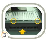
Remove the 2 screws attaching the DVD drive flap and remove the flap. If you have an existing hard drive, remove the security screw and pull on the metal handle to remove it.
