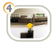
Place the Biometric FPR onto the rear of the unit, along the unit's top side.
