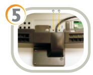
Secure the Biometric FPR to the unit using two screws from the Biometric FPR Kit.
