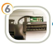
Insert the connector of the cable accompanying the Biometric FPR into the mating connector on the accessory hub in the rear of the unit.
