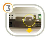
Unsecure the Biometric FPR door from the unit's top side.
