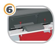
Secure wireless card module with 2 screws.
