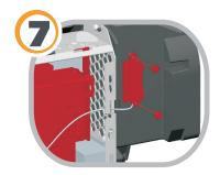
Add antenna and secure with screws.
