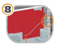
Route the antenna wire through the slot in the frame. Attach the wire to the primary connector on the wireless card.
