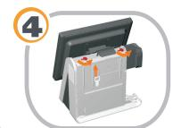
Pivot the latches to unlock the door, then lift up on the tab to remove the door.
