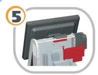
Add wireless module to top PCI connector.
