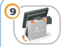
Replace the door and pivot the latches to lock it.
