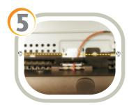
Secure the Customer Display to the unit using two screws from the Customer Display Kit.
