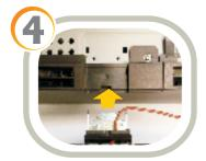
Place the Customer Display onto the rear of the unit, along the unit's top side.
