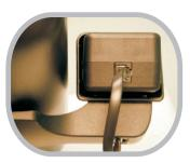
Connect one end of the RJ phone cord to the scanner and connect the other end to the cradle assembly. Place the scanner in the cradle.
