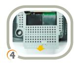
Unscrew the shielding that is connected by four screws and remove it.
