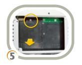
Unscrew the security screw and remove the MiniPCI cover.
