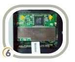
Then push the Wireless card down until it clicks. If the two side locks on the connector do not click into place, remove the card and repeat the installation until the card clicks
