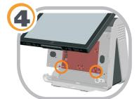
Remove the 2 screws and pull out the hard drive door.
