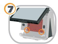
Replace the hard drive door and the 2 screws.
