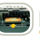
Insert the CF card into the slot. If inserted correctly, the black eject button should click and
