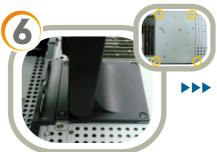
Reinstall the four screws to close the chassis and then reinstall the stand using the screws removed in Step 3.
