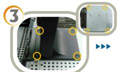
Remove the four screws connecting the stand to the chassis. Once these screws are removed, the stand will come off. Then remove the four screws on the chassis.
