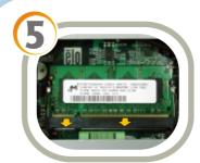
Align the pins of the memory module with the connector at an angle and push it in until the pins are in place. Then push the memory module down until it clicks. If it clicks, then it means the module was installed successfully.
