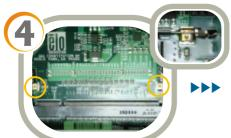
To remove an existing memory module, pull the two metal latches away from the modules until the module is released. The module should tilt up and then can be safely removed.
