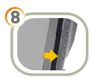
Reconnect the power adapter and power on the touchcomputer.
