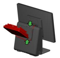
Hook the rear facing display bracket onto the AiO bracket and secure using 1 M3 screw (included in the kit) on either the top or bottom (marked by green arrows) of the bracket.
