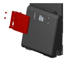
Remove the mounting screw covers from the back of the AiO and attach the bracket using the 4 screws included with the kit.
