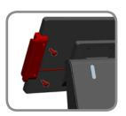
Install two new screw covers over the MSR mounting screws.
