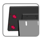
3 Secure the MSR to the back of the display as shown using the included screws.
