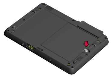
Install hand strap making sure the slotted end of the strap is fastened to the top side of the tablet. The strap can be installed for right or left handed use.
