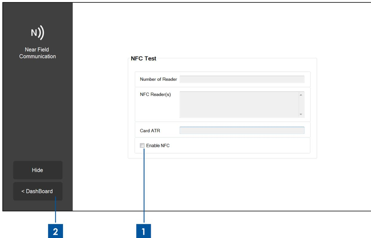
Figure 9h. NFC application of Elo Tablet Diagnostic Suite
