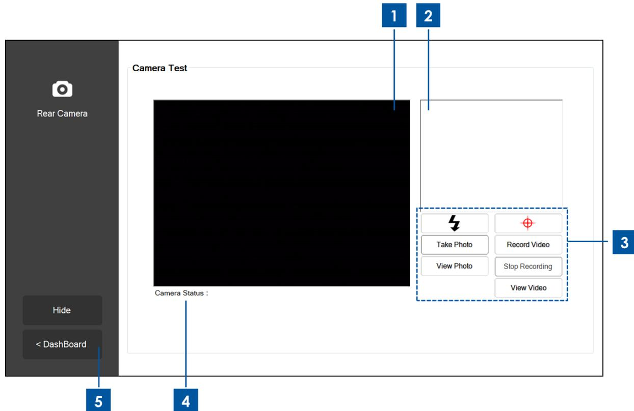
Figure 9c. Rear Camera application of Elo Tablet Diagnostic Suite
