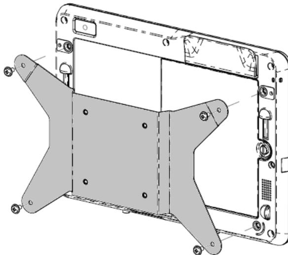
Figure 5. Optional VESA mounting bracket attaches to tablet
