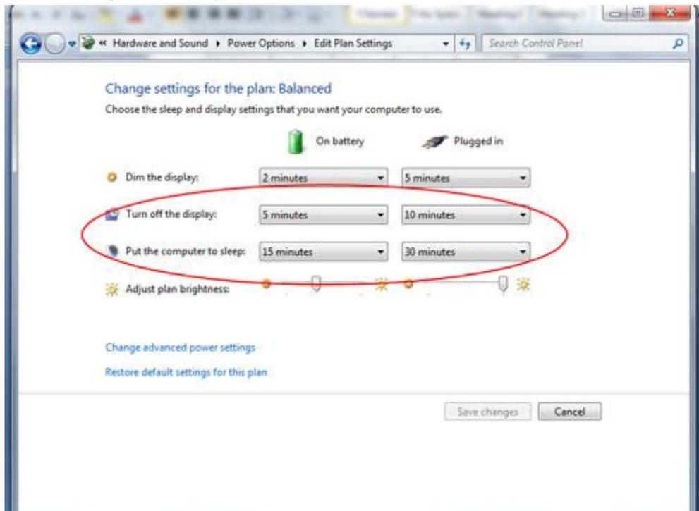
Figure 12d. The Edit Plan Setting window allows users to set the time of inactivity before the display will dim or turn off, and before the tablet will go to sleep.
