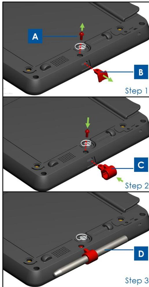
Figure 8. To install the stylus holder onto the tablet:
