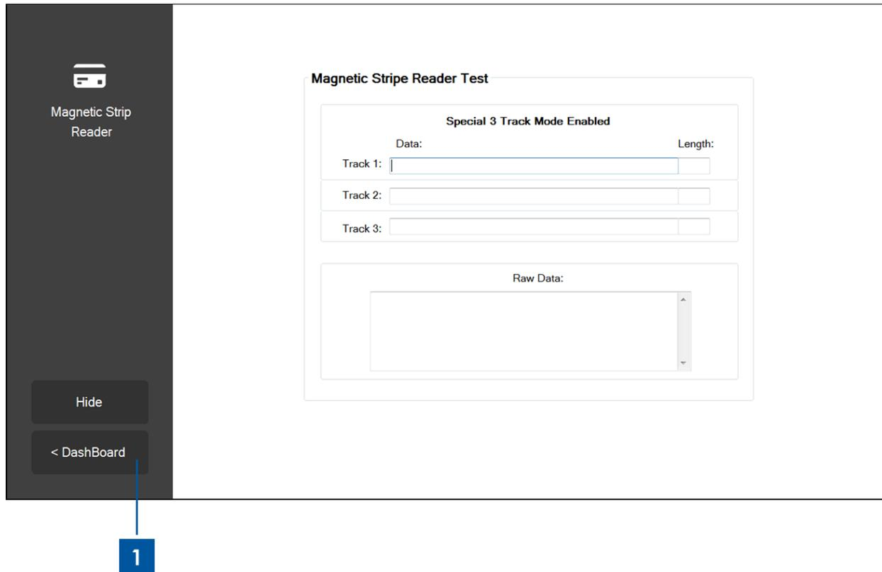
Figure 9f. MSR application of Elo Tablet Diagnostic Suite
