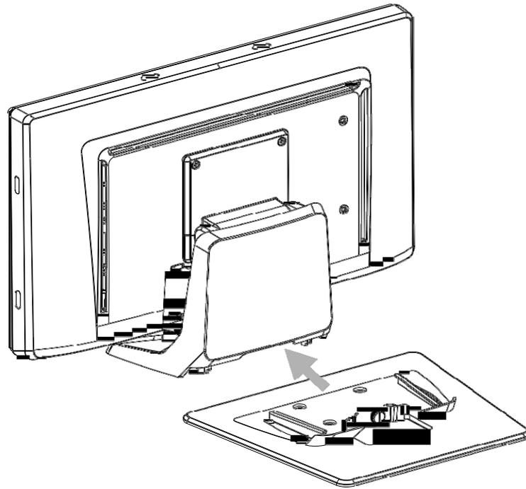
Pushing the stand plate toward the stand until it is tight, then fasten the stand plate using captive screw.
