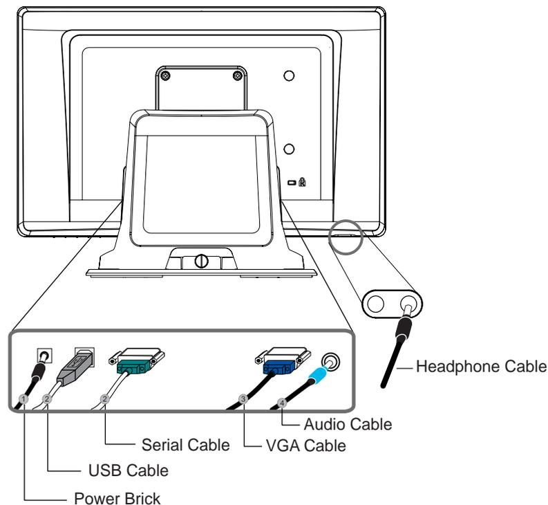
1. Connect DC cable of the power brick to the monitor and the other end through AC power cable to the AC outlet.
