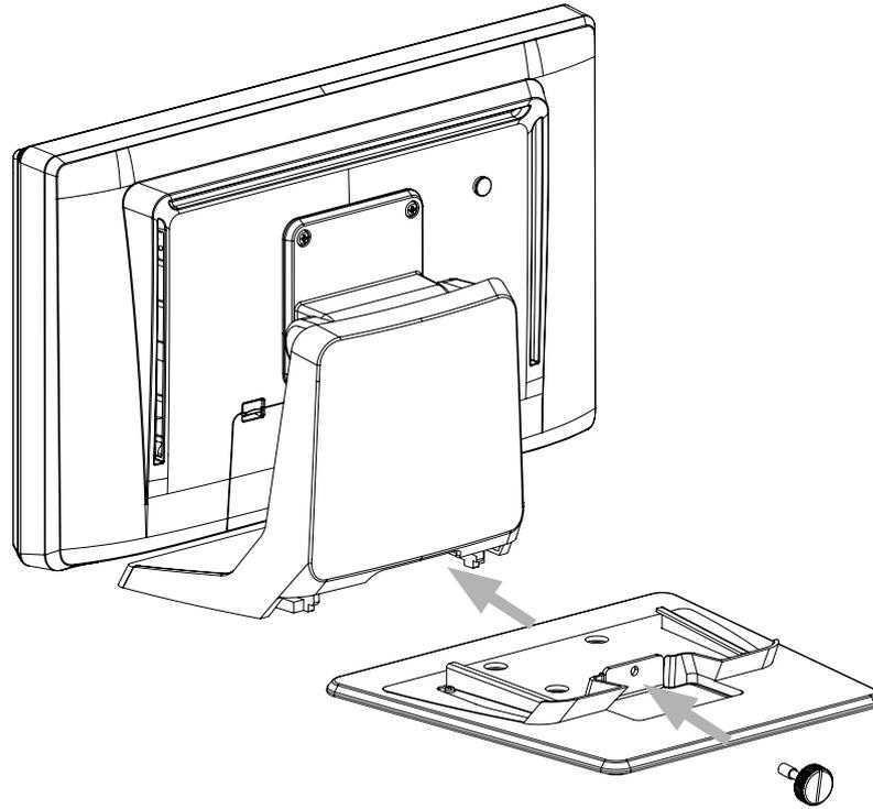
Pushing the stand plate toward the stand until it is tight, then fasten the stand plate using captive screw.
