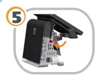
Connect the cable to the USB connector.
