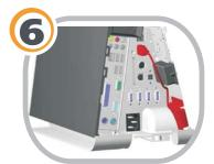
Connect the USB cable to the USB connector.
