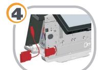
Insert the fingerprint reader module into the chassis.
