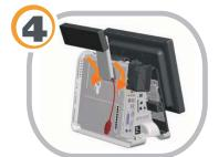
Insert the hooks on the customer display into the holes in the panel.
