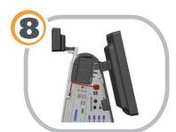
Connect the cable to the USB connector marked with the display icon.
