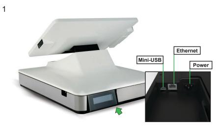
**Connect power and ethernet cables**: Connections are underneath the register near the back.
