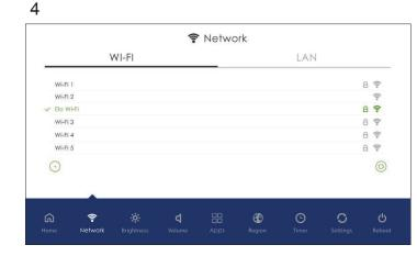
If an internet connection is not found in step 3, hold the power button down for 3 seconds and release. This lets you enter the set-up page to find your WiFi connection. Under the Network Tab, select your WiFi network. Once connected your device should start auto-provisioning itself to your software provider. Once set up is complete, password **1elo** can be used to re-enter your control panel if needed.
