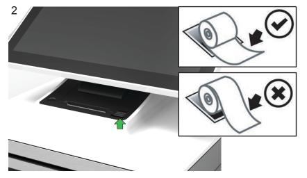
**Install receipt paper:** Install the paper by pressing the lid release button and lifting up on the printer lid. Note the correct paper orientation from the pictures above.
