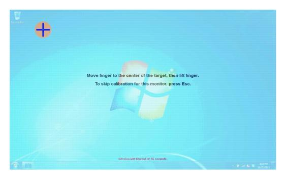
The Elo calibration tool is used to calibrate touch recognition on supported Elo touch screen monitors. After touching all 3 targets, the screen will show "Accept" and "Retry" buttons. The user can then test the calibration accuracy before selecting either "Accept" (saving calibration data) or "Retry" (re-doing the 3-point calibration).
