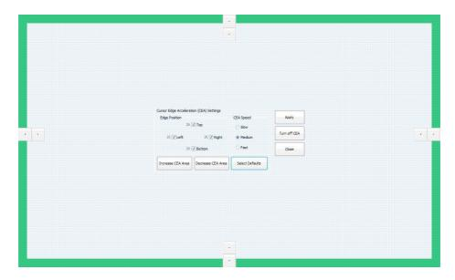
To enable CEA, click on the "Select Default" button and specify the desired parameters. The position of CEA may be manipulated for all edges at once by means of the "Increase/Decrease CEA Area" buttons, or individually by means of the arrows along each edge. Additionally, CEA for particular edges may be disabled by unchecking their respective box.
