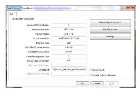
Launching "Touch Screen Properties" will display various properties of each connected (and supported) Elo touch screen such as Monitor Resolution, Controller Serial Number, Controller Firmware Version, etc. In addition to this information, users will be given the ability to "Disable Touch" and "Restore default calibration". Also in this utility are the following three advanced options:
