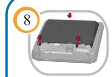
Re-install the rear cover and tighten the thumb screws.
