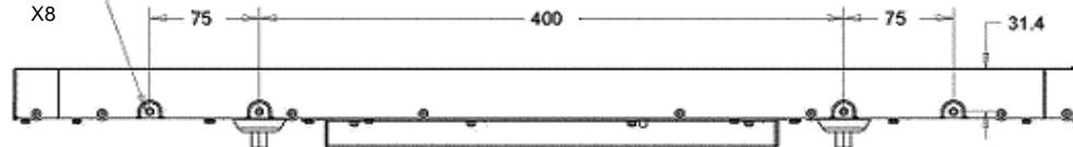
**MONTAJE LATERAL HORIZONTAL (ARRIBA/ABAJO)**
