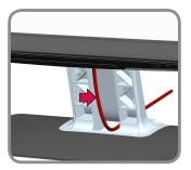
8 Optional: Install the cable clip Snap the clip over the cable and then fasten the clip to the rear of the monitor using the screw provided in the kit.
