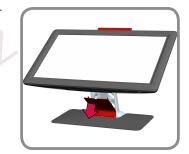
Route the periperals' USB cable through the channel in the stand and out the back.Then replace the cable cover.
