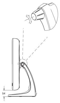
Figure 2.3 Tilt Lock Function
