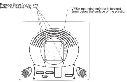
Figure 2.4 Stand and Display Separation
