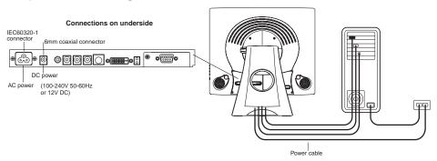
Note: The monitor is equipped with both AC and DC power connectors. The monitor is shipped with only an AC power cable.
