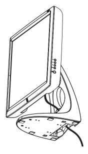
• The cables are routed through the cable management channel in the stand.
