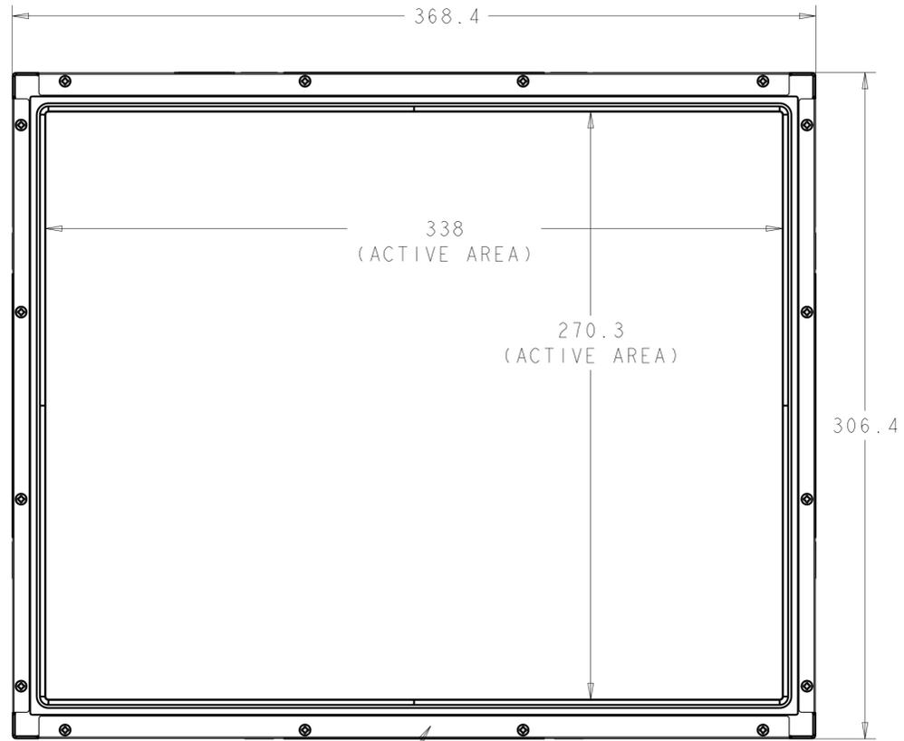
BEZEL WITH WIPER BLADE SEAL
