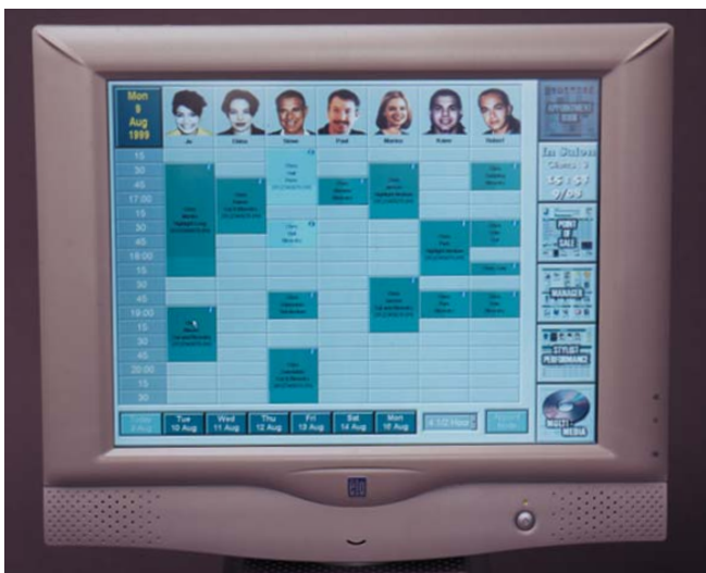
THE SHORTCUTS SYSTEM ON ELO'S 15" LCD WITH AN ACCUTOUCH TOUCHSCREEN INTERFACE IS HEAVILY USED. THE ACCURACY OF THE SCREEN WON'T DEGRADE EVEN UNDER THE KIND OF CONSTANT USE TOUCHSCREENS RECEIVE IN BUSY SALONS.
